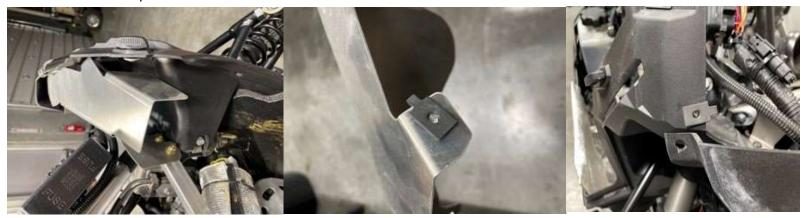
4. Remove the heat shield covering the ECU by removing the two T25 Torx screws. Then remove the ECU by removing the two 8mm bolts. Set ECU aside.
