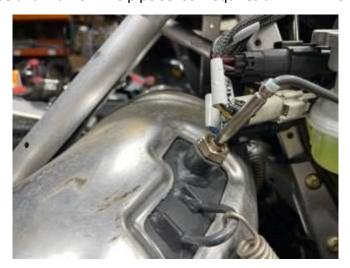
3. Remove the heat deflector. Remove the two T25 Torx screws and the 10mm nut that secure it to the sled. Remove the nut plate from the deflector and install it on the plastic piece as shown.
