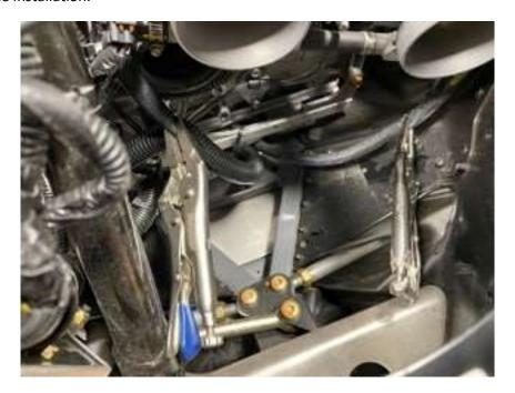
11. Install the turbo assembly into the sled. You will need to use all three stock rubber isolators from the stock muffler. You will need to trim the two brown isolators in order for them to properly fit into the turbo bracket. To trim the rubber take a razor blade and trim the side flush.
