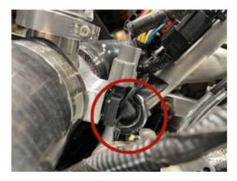
22. Install the supplied vacuum lines from the blow off valve to the vacuum ports on the throttle body.
