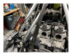
7. Remove the idle air control solenoid from the air box by removing the two T30 Torx screws and the two hoses. Remove the hoses from the throttle body and the IAC, you will not need to reinstall them. Remove the o-ring as well. Unplug the stock T-Map sensor.
