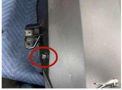
18. Install the nose piece of the hood onto the bulkhead. There are four dimples in the nose piece that line up perfectly with four holes in the bulkhead. Use four of the screws that were removed from the intake plenum to secure the nose piece to the bulkhead. This is done with ease if you have an impact drill. If you don't have one, you can do it by hand. It may be necessary to drill out the dimples first if you don't have an impact drill.
