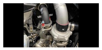
25. Install the intake tube onto the hood. Make sure the lip of the rubber connectors seal on the intake. It may take some finesse to get them seated properly. \*\*DO NOT PUT OIL ON THE RUBBER SEALS\*\*
