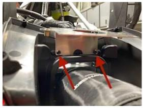
20. Install the IAC to the plastic nose piece as shown using an extra hood screw.
