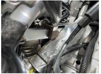
12. Install the coolant lines from the turbo to the throttle body and existing coolant hose. The coolant hose on the turbo that has the stainless splice attached will connect to the existing
