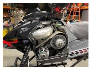
2. Remove pipe and muffler. The pipe sensor requires a 17mm wrench.
