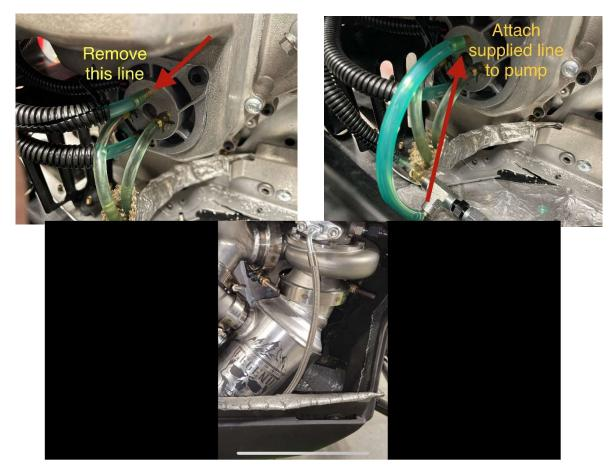
Once you have the oil hoses secured to the pump and the supplied components, make sure the braided line fittings are tight at the turbo inlet as well at the "T" side where the oil hoses connect. They should have been loose to accommodate for the oil line installation to the pump. Make sure the supply line from the pump to the turbo T is not kinked. See the picture that says, "attach supplied line to pump". That line should have a nice radius to it like pictured.
