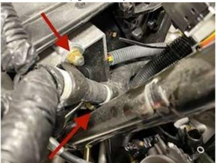
10. Before removing the coolant line from the throttle body, if you have a line clamp it is suggested that you clamp the lines to reduce the amount of coolant loss from the system. A pair of vice grips also work (just be cautious not to over clamp the lines as they could be cut). Remove the line from the throttle body on the right (mag) side. Do not lose the clamp as you will need this for the installation.
